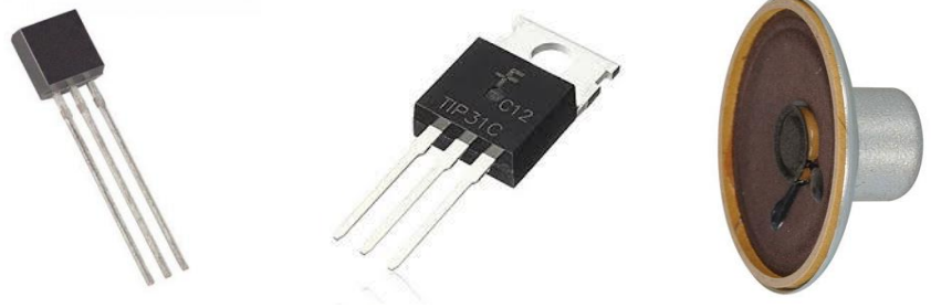
Fig. 0: (Left) Small signal BJT (Center) Power BJT (Right) Audio speaker.
